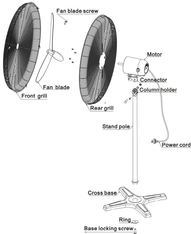
1. Unscrew the base locking screw and ring from the stand pole and bang the stand pole through the hole in the center of the cross base.
