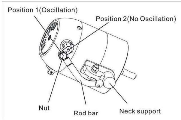
The diagram above shows the underneath of the fan's Motor unit. In the position shown, ie. Position 1 (Oscillation), the fan head will swing side to side during operation. To fix the fan head to blow air in a fixed direction, first turn off and unplug the fan, then unscrew the 'Nut' and screw it into the other hole – Position 2 (No Oscillation).
